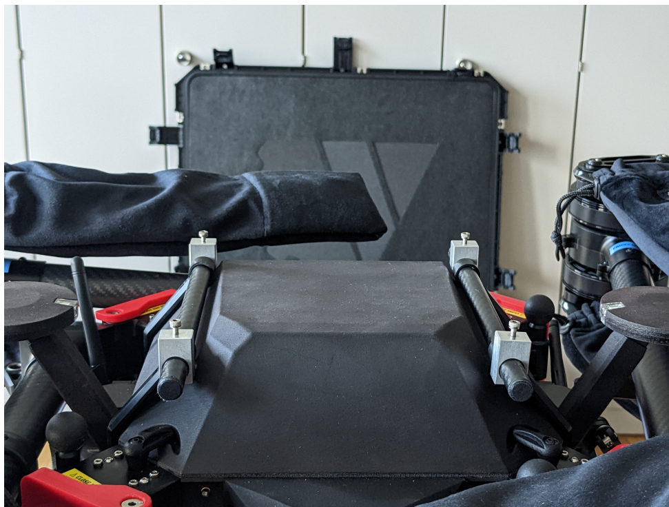
Figure 21: Mounting points for the adapter plate of the Prism Coaxial X8
