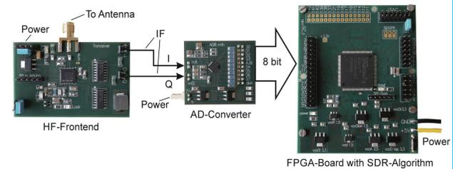
Fig. 8: Receiver Breadboards without  $\mu$ Processor
