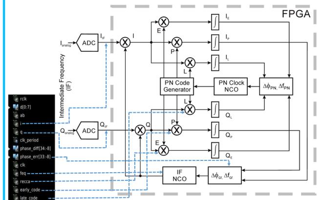
Fig. 9: Flow chart of receiver FPGA module
