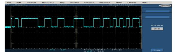
Fig. 7: Measured base band PN signal
