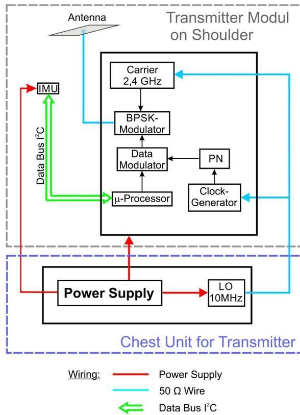
Fig. 3: Transmitter for Shoulder
